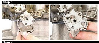
Install the back plate section of the linkage adapter. Take care as to not bend or tweak to long thin side of the back plate. Notice the pre-drilled and tapped hole in the middle of the back plate. This is important for the next step.
