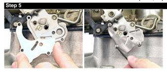
Position the front face plate of the linkage adapter over the linkage as shown in the picture on the left. Now fasten the front plate to the back plate using the provided 6/32" X 3/8 and 6/32" X 1/4" screws and the 5/64" Allen wrench.
