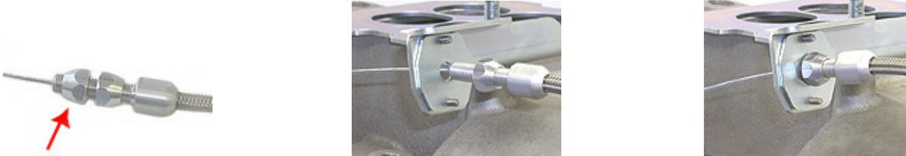
Remove the first adjuster nut, the one indicated by the red arrow in the above left picture. Position the second adjuster nut on the threaded cable housing so the adapter plate will be in the middle of the threaded areas once it's installed into the adapter plate. Slide the cable adjuster housing through the hole in the adapter plate as shown in the pictures at upper right and below left.
