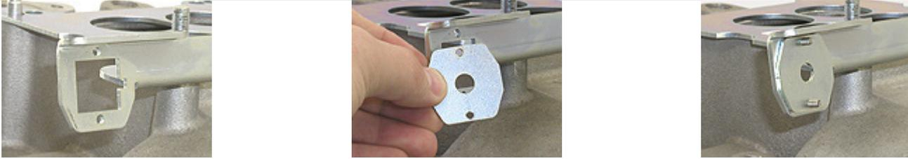
Install the stainless steel braided cable adapter piece provided in the TV Made EZ kit. This adapter must be mounted on the back side of the base plate bracket as shown in the pictures above. Secure the adapter to the base plate bracket with the provided 6-32 stainless steel pan head screws and Allen wrench.
