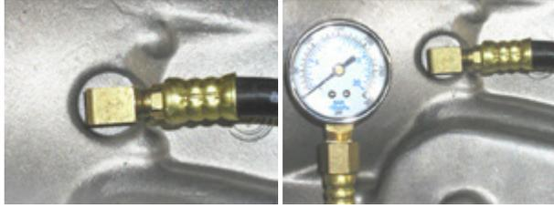
Screw the pressure gauge hose into the 90 degree fitting. Be sure that it's snug inside of the fitting to prevent leaking. Route the pressure gauge hose above the frame and away from the exhaust. You can now use the gauge under the hood or while test driving, routing up through the driver side window.. That's it! We don't recommend this gauge be installed permanently, it should be removed after the set up and test driving are completed.
