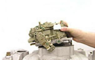
Remove the carburetor and gasket from the manifold. Make sure that the gasket surfaces are clean before you proceed to the next step.
