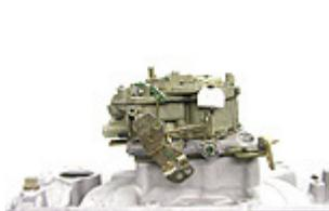
Put your carburetor back on the manifold. Reconnect all the hoses, wires and linkage disconnected when removing the unit. Tighten the hold down nuts evenly using a cross pattern; applying a little more torque each sequence. This procedure will prevent damaging the carburetor.
