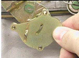
Position the front face plate of the linkage adapter over the linkage as shown in the picture on the left. Now turn the face plate until the four bolt holes line up with the back plate section installed in the previous step.
