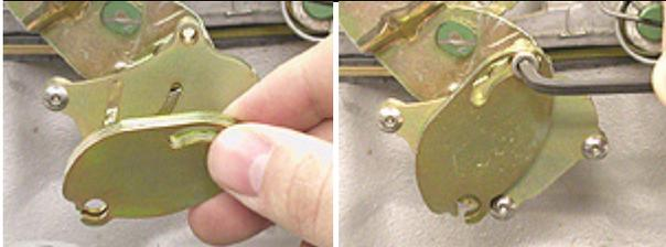
Align the roll pins on the back side of the cam into the slots on the linkage adapter face plate. Once the cam is indexed correctly, install the 8/32" cap screw and tighten using the provided 9/64" Allen wrench. Again be careful not to over tighten this small screw.
