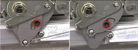
You are ready to perform your test drive! We recommend the pressure gauge remain hooked up during all test driving. Pay attention to the reactions caused by the TV system, it is very educational. During the test driving we also recommend allen wrench supplied in the TV Made EZ kit that fits the cap screw shown within the red circles at left. Start with the cam in the lower position (far left picture), perform a test drive while making mental notes of the shift timing and feel characteristics.
