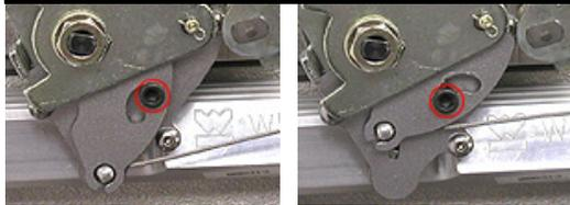
We strongly recommend you leave the pressure gauge hooked up during all test driving. It is very educational to observe the operating pressure reactions caused by the TV system. During the test driving we also recommend taking along the Allen wrench supplied in the TV Made EZ kit that fits the cap screw that holds the cam from moving. (Like the one shown within the red circles at left) We recommend you start with the cam in the lower position (far left picture), Perform a test drive while making
