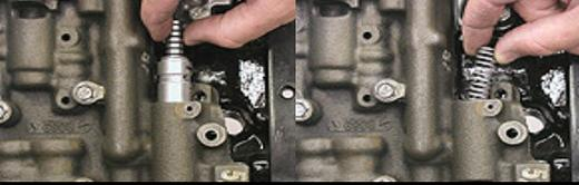
You will then need to remove the TV Plunger and the bushing. To do this, simply pull the TV plunger and bushing out. Now remove the old spring. If the TV plunger and bushing prove difficult, you can make the TV plunger act as a slide hammer by simply pushing it all the way in, release it in such a way as to cause it to "snap" back out, repeat this action as necessary until you get it removed.
