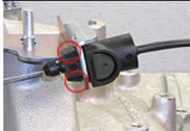
Check that the two retaining "tabs" on the TV cable housing have spread out and locked the cable into the base plate bracket. These tabs prevent the cable housing from coming out. (Red circles at right)
