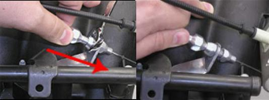
Now that you have your braided TV cable installed on your bracket, you have to adjust it. Start by loosening the back adjuster nut using a 10mm (1/2") wrench. At the same time, push on the cable housing as to move it forward. You will want to keep moving it forward until you see the pressures on your pressure gauge stop decreasing.
