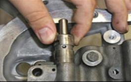
You will then need to remove the TV Plunger and the bushing. To do this, simply pull the TV plunger and bushing out. Now remove the old spring. If the TV plunger and bushing prove difficult, you can make the TV plunger act as a slide hammer by simply pushing it all the way in, release it in such a way as to cause it to "snap" back out, repeat this action as necessary until you get it removed.
