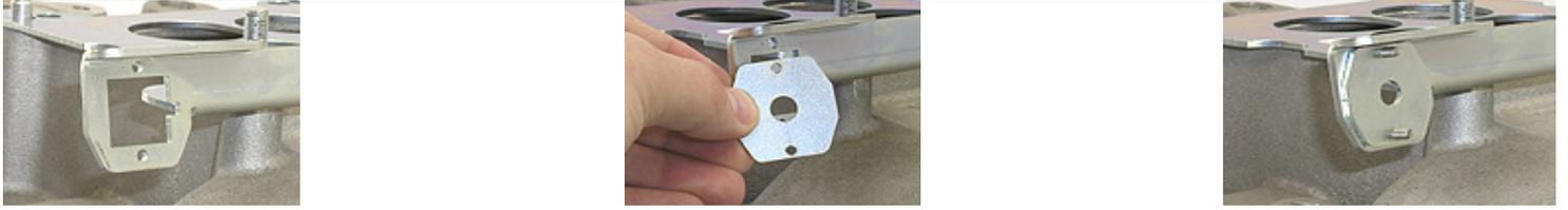
Install the stainless steel braided cable adapter piece provided in the TV Made EZ kit. This adapter must be mounted on the back side of the base plate bracket as shown in the pictures above. Secure the adapter to the base plate bracket with the provided 6-32 stainless steel pan head screws and Allen wrench.
