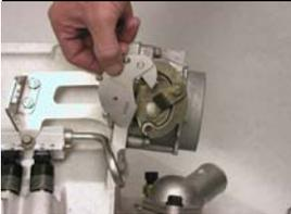
Replace the stock linkage assembly with the linkage assembly supplied and install it on the throttle arm.
