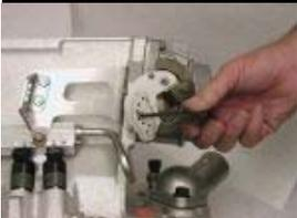
Install the cam assembly to the linkage assembly and fasten with the 8-32 x 5/8 SHCS
