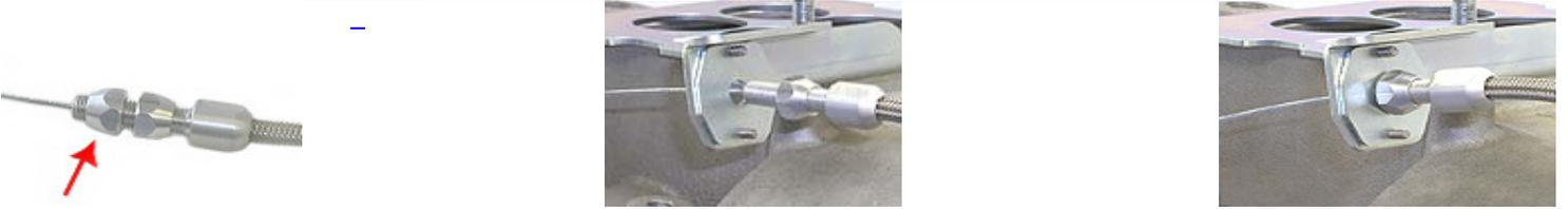
Remove the first adjuster nut, the one indicated by the red arrow in the above left picture. Position the second adjuster nut on the threaded cable housing so the adapter plate will be in the middle of the threaded areas once it's installed into the adapter plate. Slide the cable adjuster housing through the hole in the adapter plate as shown in the pictures at upper right and below left.
