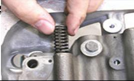
**TV Made Ez - 700R4 Spring replacement and shim installation guide sheet**
