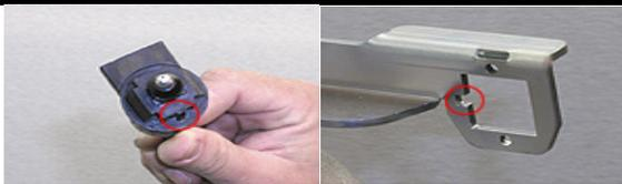
Insert the TV cable into the base plate bracket until you hear it click into position. To do this, match the index guide on the TV cable housing, with the notch in the base plate bracket (red circles in the pictures). The cable will not go in any other way.
