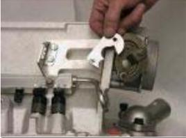
Remove the stock GM linkage assembly.
