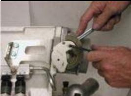
Fasten the Linkage assembly with the 1/4-20 fastener and the 1/4-20 lock nut into the mounting hole.
