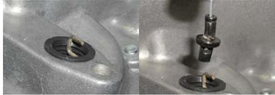
The TV cable is connected to the passenger side of Th-2004R and Th-700R4 transmissions at the locations shown in the above pictures. Same side as your dipstick. The picture at the far left shows the wire link and the TV cable to case seal. This seal must be placed into the transmission before installation, not onto the end of the TV cable housing! The wire link will be inserted into the hole of the connector at the transmission end of the TV cable.
