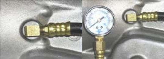
Screw the pressure gauge hose into the 90 degree fitting. Be sure that it's snug inside of the fitting to prevent leaking. Route the pressure gauge hose above the frame and away from the exhaust. You can now use the gauge under the hood or while test driving, routing up through the driver's side window. That's it! We don't recommend this gauge be installed permanently, it should be removed after the set up and test drive are completed.
