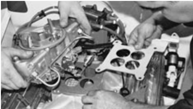
Since someone didn't want to pull the fuel line off, we employed an extra set of hands to help out with the quick exchange. Make sure there is no residual gasket material on either the carb base or manifold before reinstalling the carburetor. It takes a gasket on each side of the TV cable carburetor plate. Wow, that's a mouthfull.
