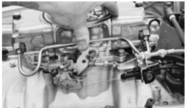
The next step is to manually rotate the carburetor linkage to W.O.T. (wide open throttle). However, as you attempt to rotate the carb linkage the TV cable will add drag to this action. You must force the throttle open all the way, causing the TV cable slider mechanism to ratchet out to its correct set position. You will hear the ratcheting sound to let you know it has been set. This establishes the correct wide-open throttle relationship between three key components in the TV system, and completes the set-up procedure. This set position will automatically establish the correct working relationship between the cable and transmission.
