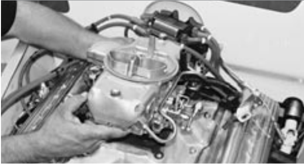
Remove the accelerator cable, fuel line, choke wire, and the four carb bolts.
